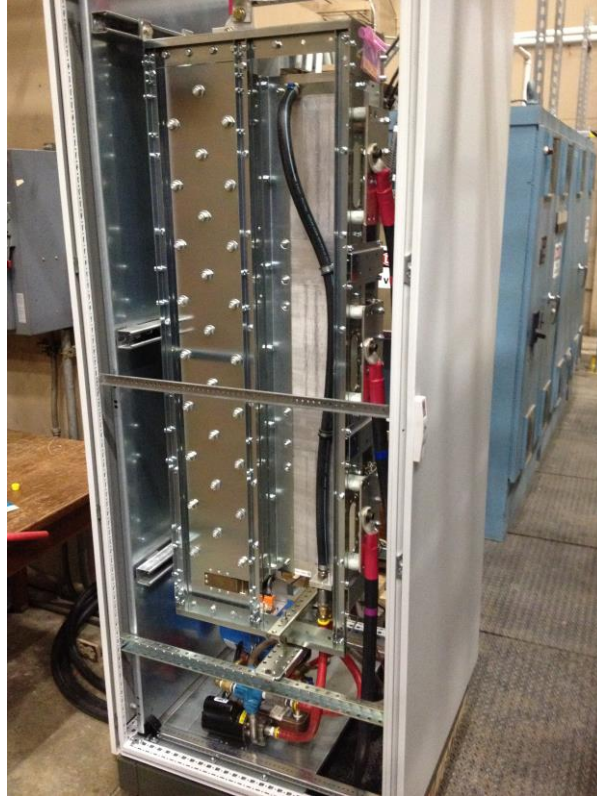
Figure 1. Semikron Semistack RE half-bridge module connecting the dc bus to the PFN charging power supply.
