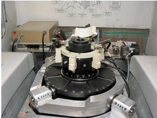
Transit Bus Flywheel 150-250 kW (peak), 100 kW (cont.), 2 kW-h
