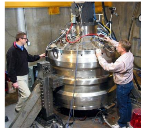
Advanced Locomotive Propulsion System Flywheel 3 MW (peak), 2 MW (cont.), 130 kW-h
