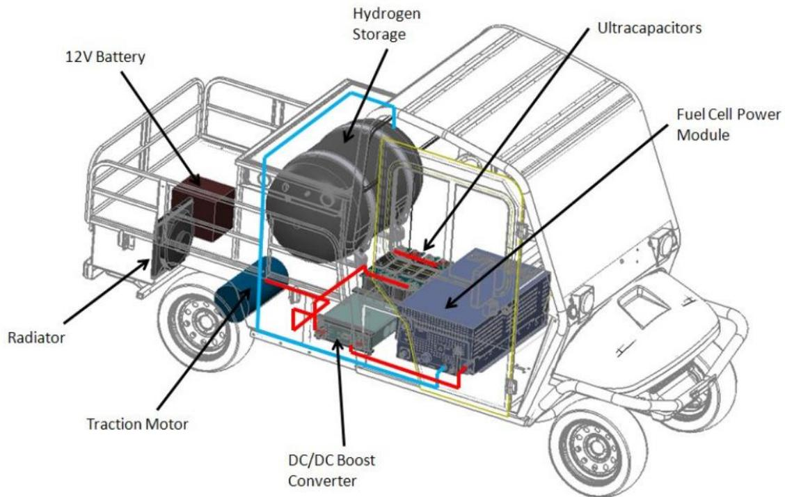
**Figure 1. Layout of integrated components**
